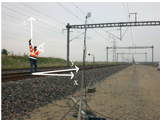
FIG. 1. (Color online) Position of the acoustic source (alarm pistol) on the experimental site.
