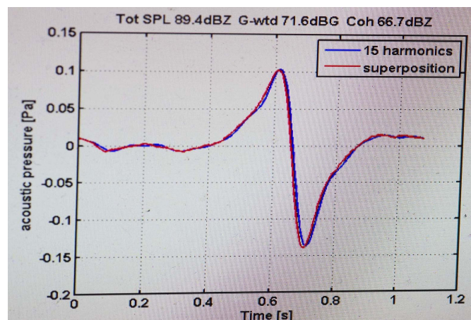
Figure 10 [63]: An infrasonic pulse extracted from the emission of a wind turbine. The fluctuations of sound pressure measurable near a wind installation usually contain noise, i.e. , irregular sound events of different origin. Noise removal is possible by averaging the sound pressure over a large number of mast-blade passages (here 4100), which reveals their common element (red line). The red peak thus visualized from the time sequence coincides
